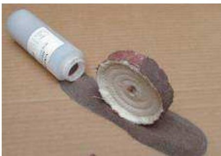
Finally, roll the wheel into the abrasive using light pressure, ensuring a heavy pickup of the abrasive.
