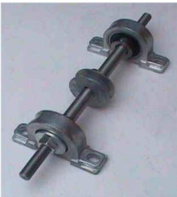
**BENCH MANDRELLS** are an inexpensive way of making up a special buffing machine. The shaft ends are ½” diameter are left and right hand threaded. The Chuck adapter can also be screwed onto one end of the mandrel, allowing the operator to attach flap wheels, sanding drums and felt bobs.
