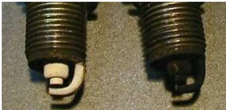
The brownish color over the tip and part of the center porcelain on the left plug indicates a carb with proper mixture. The uniform more whitish color of the right plug indicates a carb that the mixture is still a little lean.
