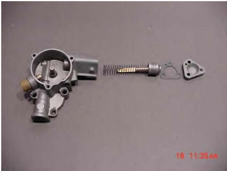
· Unscrew the brass breather plug from the housing. The enrichment needle can be removed through this hole.
