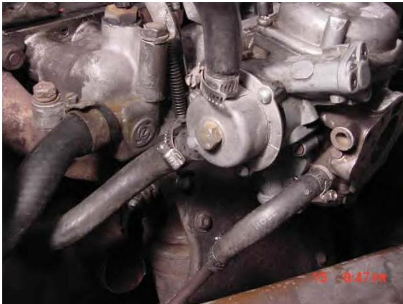
You will probably have to fool with the fast idle and the slow idle screws to get them set correctly. Also, you may find that lining up the index marks may result in a mixture too lean or too rich for starting and cold running. To adjust, loosen the three screws that hold the heat mass, and rotate the heat mass counter clockwise to lean the mixture, and clockwise to richen it. Don't turn too much....a little goes a long way. If everything is working right, the
