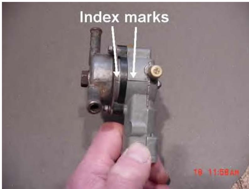
· Reconnect the hoses to the heat mass, making sure you don't rotate the heat mass while doing so.
